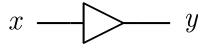
Reversible Computing, Figure 3 A unit wire, which acts as a delay element ( y(t) = x(t - 1) )
