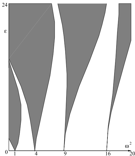
Perturbation Analysis of Parametric Resonance, Figure 1 Floquet tongues of the Mathieu Eq. (15); the instability domains are shaded
