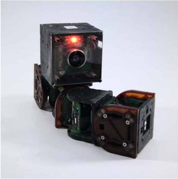
Modular Self-Reconfigurable Robots, Figure 4 CKbot module cluster. 4 CKbot modules and one CKbot camera module are joined together in a cluster. Several clusters can join together attaching magnetically
