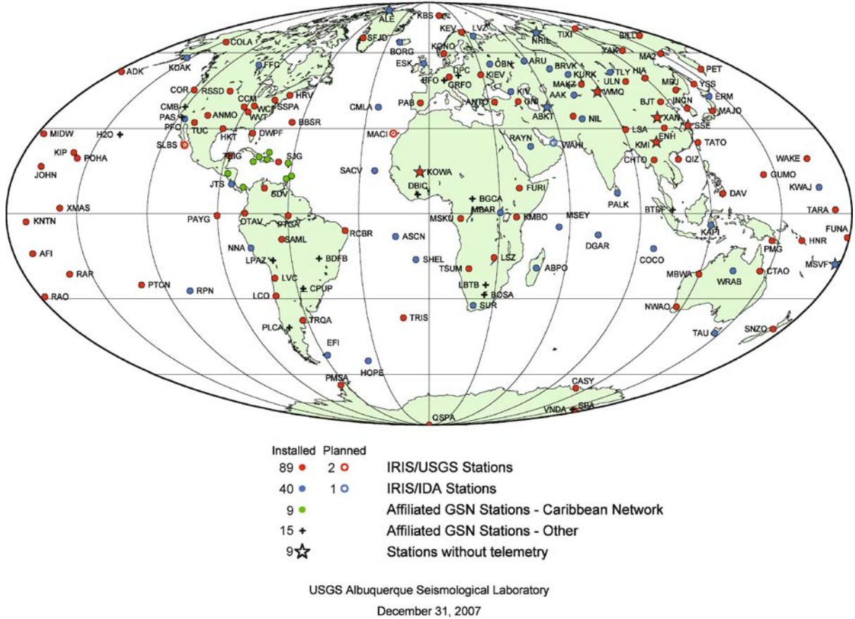
Earthquake Monitoring and Early Warning Systems, Figure 10 Station map of the Global Seismographic Network (GSN) as of 2007
