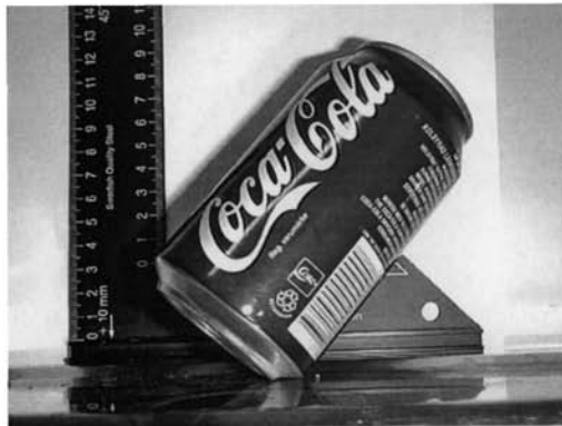
Figure 4.5-1. The balance of a tilted Coca-Cola can.
