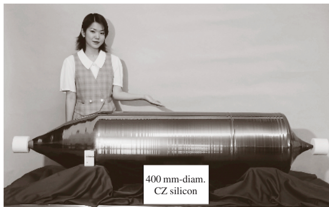
Fig. 13.8 Extra-large as-grown Czochralski silicon ingot 400 mm in diameter and 1800 mm in length. (Courtesy of Super Silicon Crystal Research Institute Corporation, Japan)
