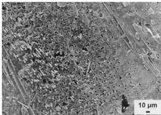
Figure 8. SEM micrograph showing a typical fracture surface of a composite after 20 thermal shock cycles
