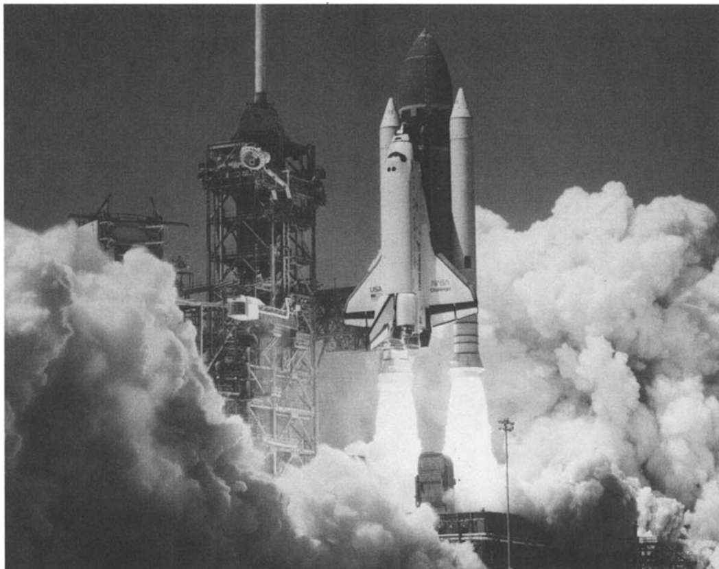
Fig. 37.18. The solid booster rockets for the space shuttle are one of the most widely publicized applications of solid rocket propellants.
