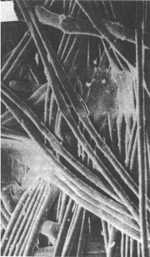
Fig. 12.22. Spunbonded polypropylene showing interfiber bonding, which binds the structure. (Courtesy E. I. DuPont de Nemours & Co.)
