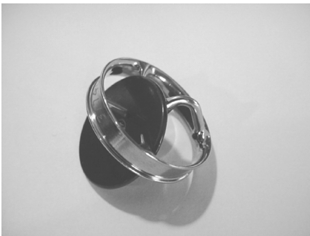
Fig. 6.1. A typical PyC leaflet heart valve (Medtronic)
