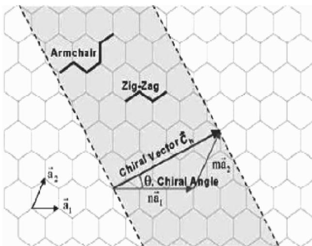
Fig. 12.4. Unit cell of a carbon nanotube
