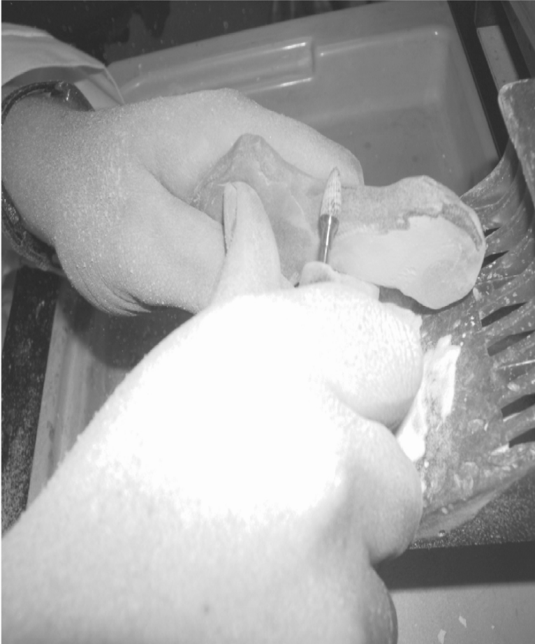
Fig. 8.8. Grinding of light curing polymer, note method of holding handpiece and dust generated
