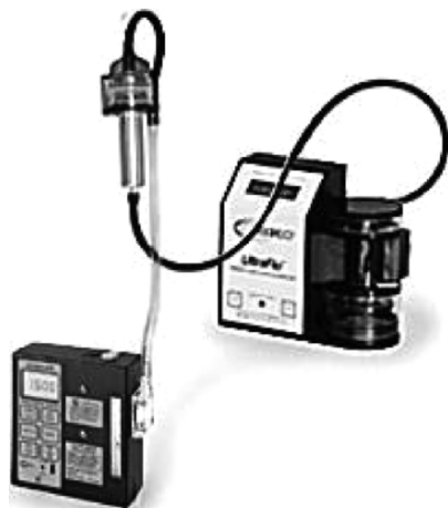
Fig. 10.7. Personal sampler used to monitor for respirable dust (Permission: SKC, Inc.)
