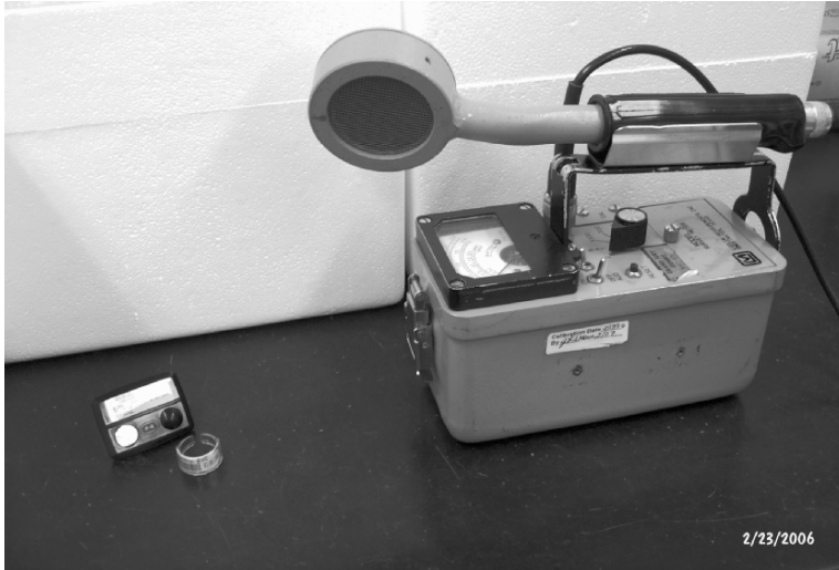
Fig. 10.15. Radiation dosimeter (left) and Geiger-Mueller counter for radioactivity surveys
