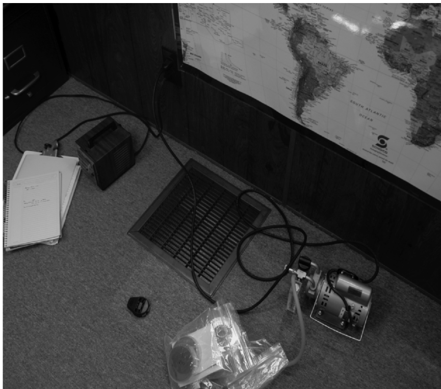
Fig. 10.18. Viable contaminant monitoring apparatus with agar plates
