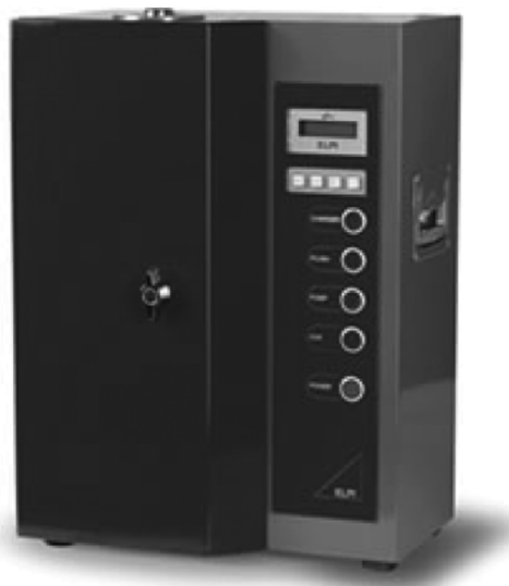
Fig. 10.9. Electrical Low Pressure Impactor (Permission: Dekati, Ltd.)
