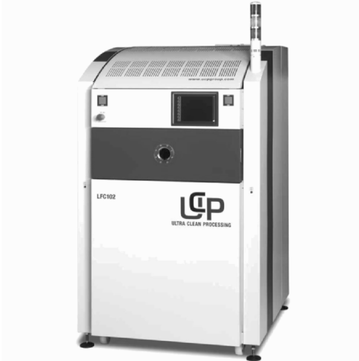
Fig. 10.4. Plasma cleaning apparatus (Permission: UCP Processing Ltd)
