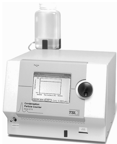
Fig. 10.8. Condensation particle counter (Permission: TSI, Inc.)
