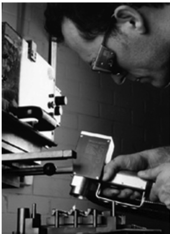
Fig. 10.5. Laser cleaning operation (Permission: Adapt Laser Systems)
