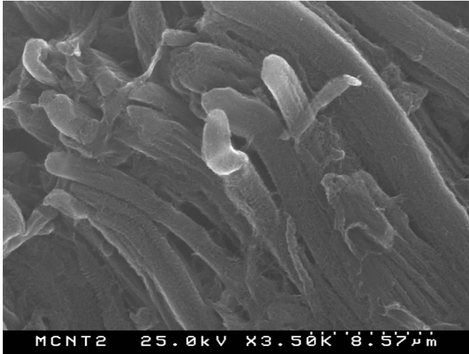
Fig. 12.6. As-grown CNTs in bundle form synthesized using the microwave plasma (MP) CVD method
