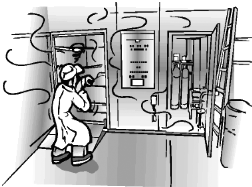
Fig. 10.2. Illustration of ethylene oxide (EtO) leaking from a sterilization chamber (Permission: Japanese Advanced Information Center for Safety and Health)
