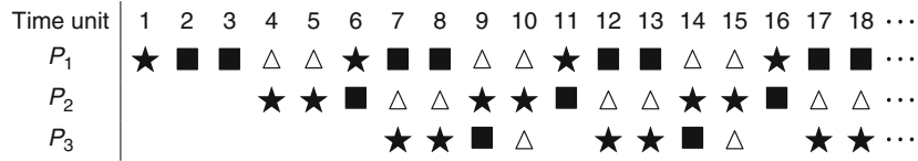
Task Graph Scheduling, Fig. 10 An example of one-to-one mapping with three stages and processors. Each processor periodically receives input data from its predecessor (★), performs some computation (■), and outputs data to its successor (△). Note that these operations are shifted in time from one processor to another. The cycle-time of P_1 and P_2 is 5 while that of P_3 is 4, hence T_{\text{period}} = 5
