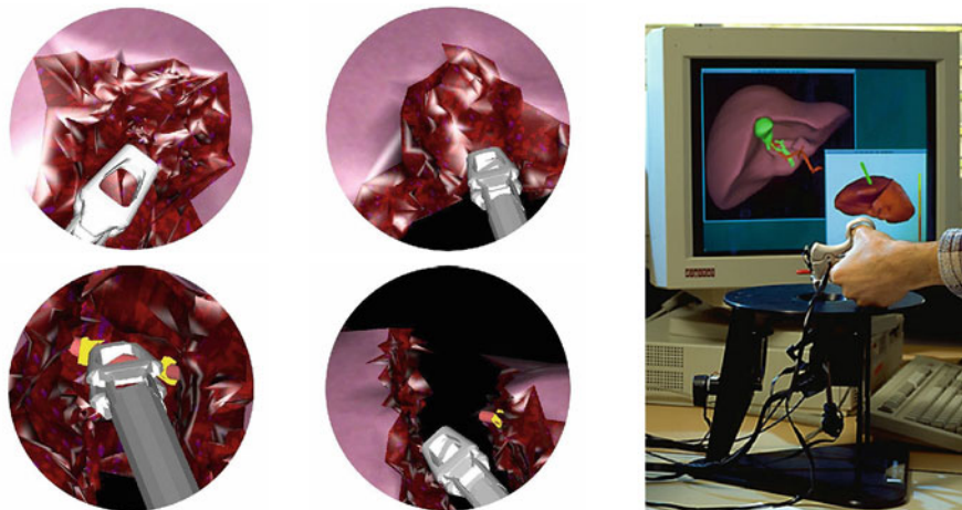
Fig. 3 (Left) View of the simulated hepatic resection involving linear-elastic materials (from [12, 13, 15] and [20, 21]); (Right) A force feedback system suited for surgery simulation
