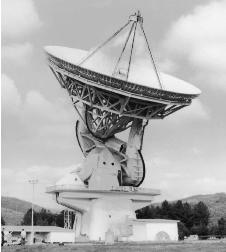
Fig. 1.6 The 140-ft. (42.6-m) diameter, equatorial radio telescope at the Green Bank, WV, facility of the US National Radio Astronomy observatory. The telescope saw first light in 1964 and was taken out of service in 1999
