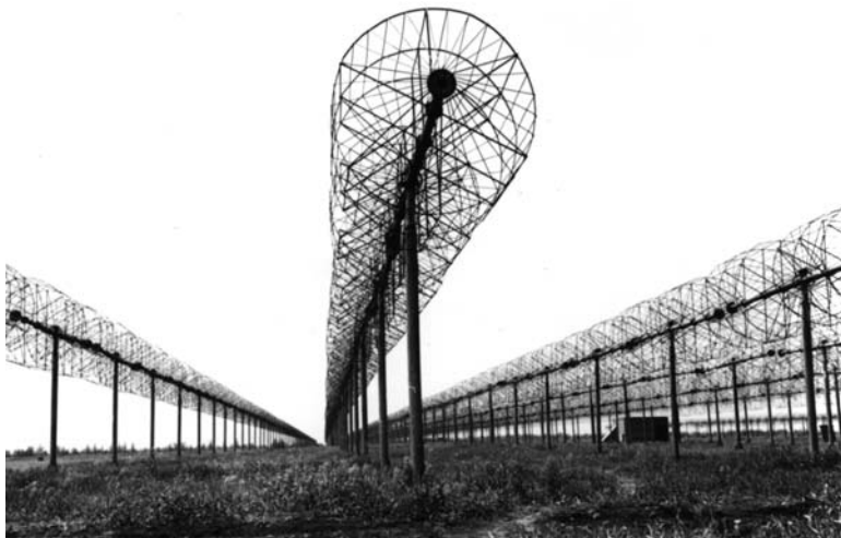
Fig. 2.32 The 1,800 \times 900 m UTR-2 radio telescope of the Radioastronomical Institute of the Ukraine at Kharkov. With this instrument, the longest wave carbon RRLs were detected at decameter wavelengths
