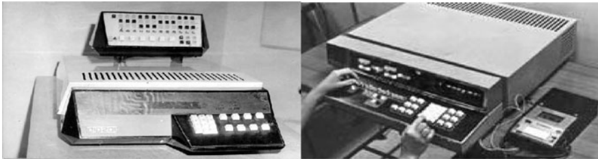
Figure 1 First Cuban minicomputer. Left hand: Prototype CID 201. Right hand: Serial model CID 201A.
