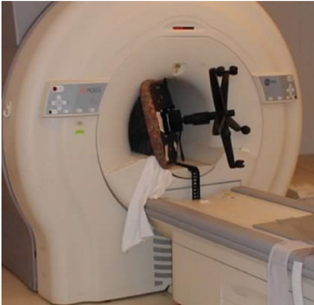
Fig. 33.1 Non-MR conditional chair attracted to magnet
