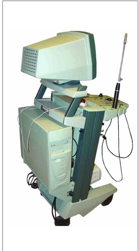
Fig. II.13. Hardware (BK 3Di) for acquisition, reconstruction, and visualization of three-dimensional ultrasound images
