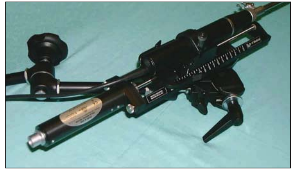
Fig. II.14. Ultrasound probe type 1850 and colorectal pull-back mover (UA0552) used to acquire three-dimensional anorectal endo images (a, b)
