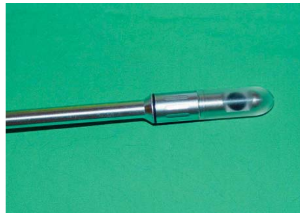
Fig. 5. The end of the probe is covered with a plastic cone
