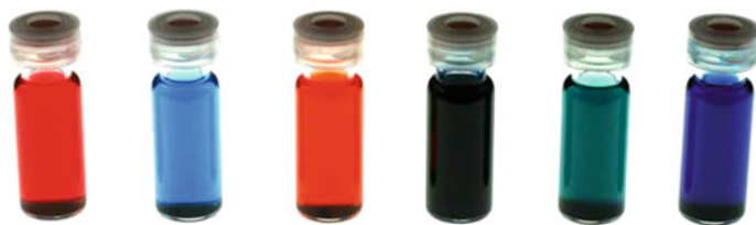
Fig. 5 Examples of some azo dyes (from left to right): Sudan IV (staining of lipids), Evans Blue (dye for immunofluorescence), methyl red (pH-indicator), Sudan black (staining of lipids), Sudan green , and basic aniline dye methylene blue (stains parasitic protozoa like plasmodia)
