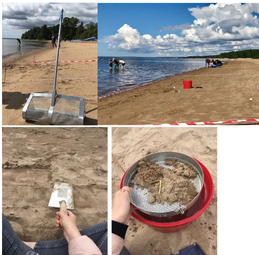
Fig. 2 Application of Frame and Rake methods on the beaches of the Neva Bay (photo by A. Ershova)
