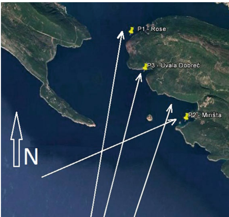
Fig. 17 Illustration of exposure of suitable mariculture sites to waves from the open sea (Source: modified from Google Earth)
