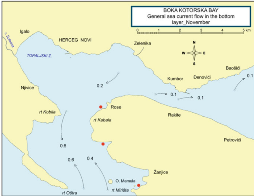
Fig. 12 General sea current flow at a bottom layer for the month of November (velocities in knots) with marked potential aquaculture sites (red dots), modified from [29]
