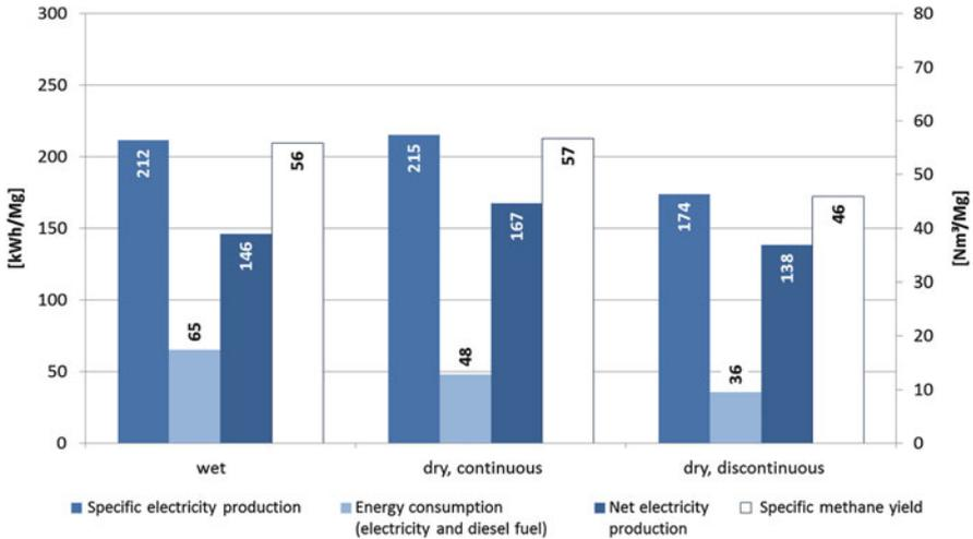
**Fig. 5** Comparison of electricity production, consumption, and net electricity yields of wet and dry processes for anaerobic treatment of biowaste and green waste relative to the input into the facility
