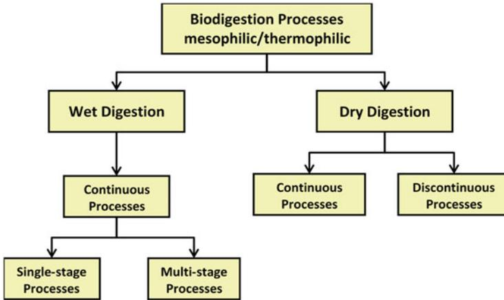
Fig. 3 Types of anaerobic treatment technologies and processes
