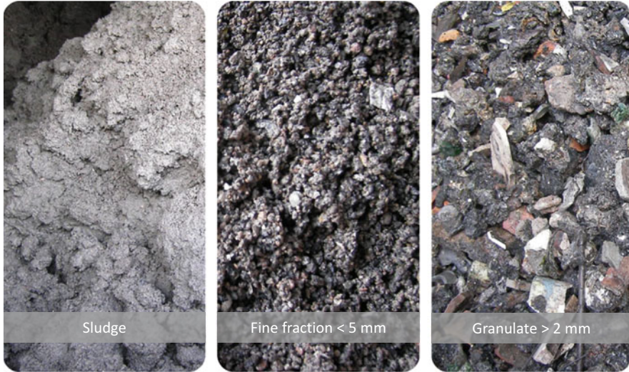
Fig. 9 Granulate product from SYNCOM-Plus process ( right ) and sludge, as well as fine fraction for recycling in the incineration process (Photos Peter Quicker)
