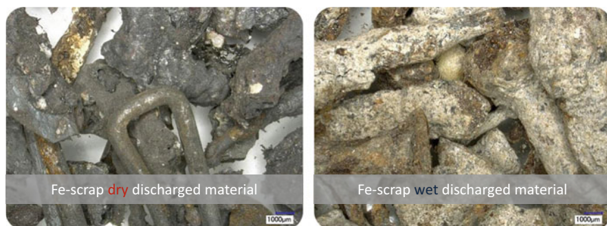
Fig. 11 Iron product from dry ( left ) and wet ( right ) discharge of MSWI bottom ash
