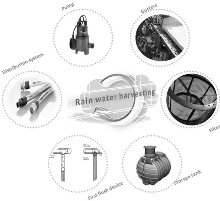
Fig. 18 Most used rainwater harvesting system parts [12]
