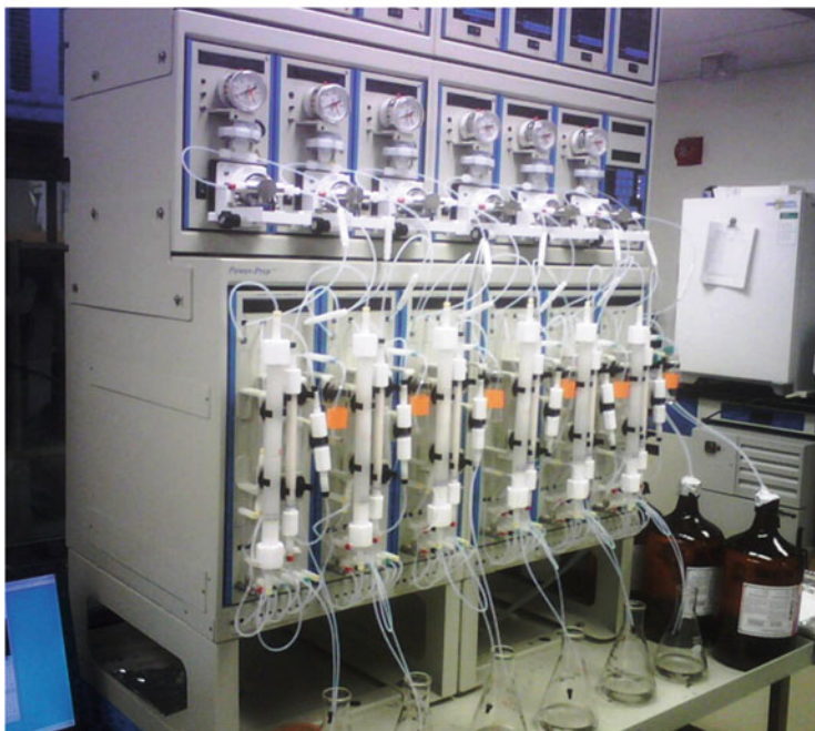
Fig. 2 (a) Schematic representation of an automated cleanup system. Reproduced with permission from [76] of GC-MS. (b) FMS PowerPrep System
