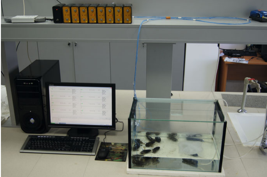
Fig. 4 Experimental unit for cardiac activity recording of aquatic invertebrates
