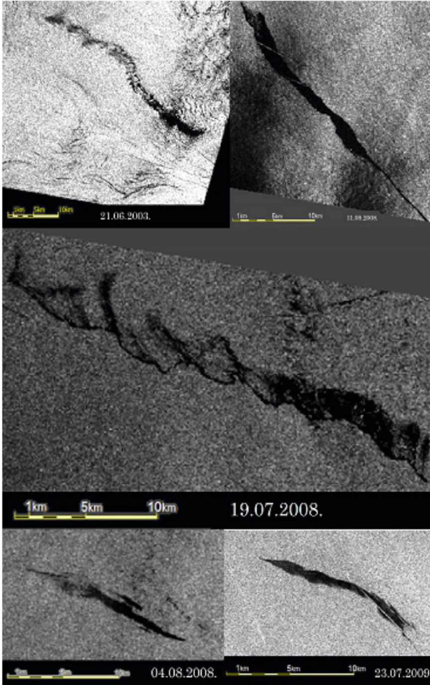
Fig. 7 Subscenes of Envisat SAR images of 21.06.2003, 11.09.2008, 19.07.2008, 04.08.2008 and 23.07.2009, with very large slicks, which are definitely ship-made oil spills. © ESA
