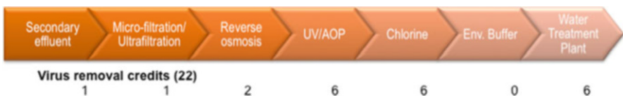
Fig. 3 Virus log removal efficiency by a potable water reuse treatment train consisting of integrated membrane systems followed by advanced oxidation processes and an environmental buffer
