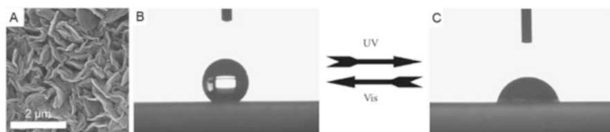
Fig. 17 SEM images of the top and cross section views of the hybrid of \text{CF}_3\text{AZC}_5\text{COO}^- intercalated ZnAl-LDH (a) and shapes of a water droplet on the hybrid film surface (b) before the UV irradiation and (c) after the UV irradiation (Reproduced from the reference [427] with permission)
