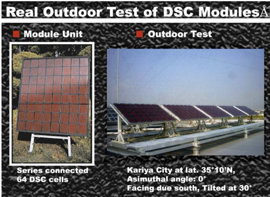
Fig. 22 Outdoor field tests of DSC modules in Kariya City Japan at lat. 35°10'N, Azimuthal angle 0°, facing due south, tilted at 30°. Note the pc-Si modules in the second row
