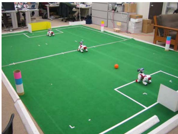
Fig. 4. Initial position for each experimental trial. The three robots are placed in three positions on the field, with the ball in the defense area. The experiment proceeds until the robots advance the ball past the end line of the opposite half of the field.
