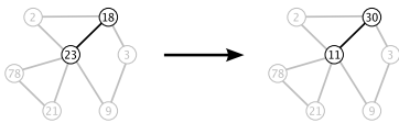
Fig. 1. Vertices represent robots and edges communication links. Numbers depict Process 1 state. A random value (12 here) is exchanged. No state information in gray is necessary, it is a strictly local interaction.
