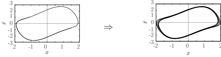
Fig. 5b. Convergent shift by structural transition
