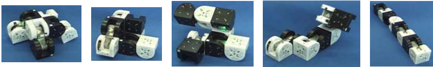
Fig. 4. Metamorphosis from a four-legged walker to a linear form.
