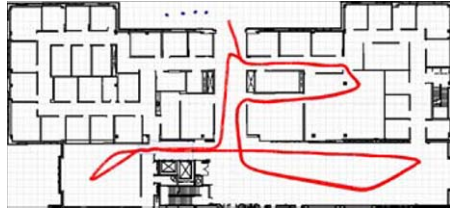
Fig. 3. Floor plan with initial robot positions and firefighter path. Initial position of the firefighter is the topmost point of the path.
