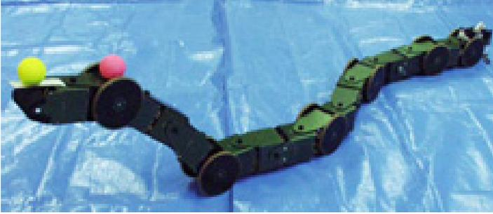
**Fig. 4.** A research platform robot (ACM-R3)
