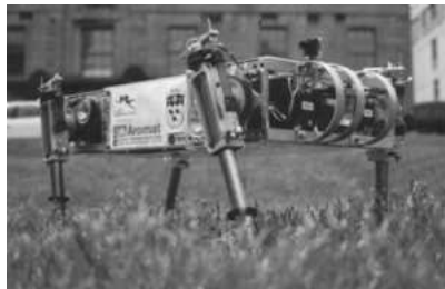
Fig. 1. Scout II: A simple four-legged robot.
