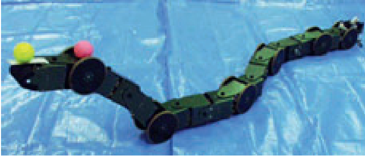
Fig. 4. A research platform robot (ACM-R3)
