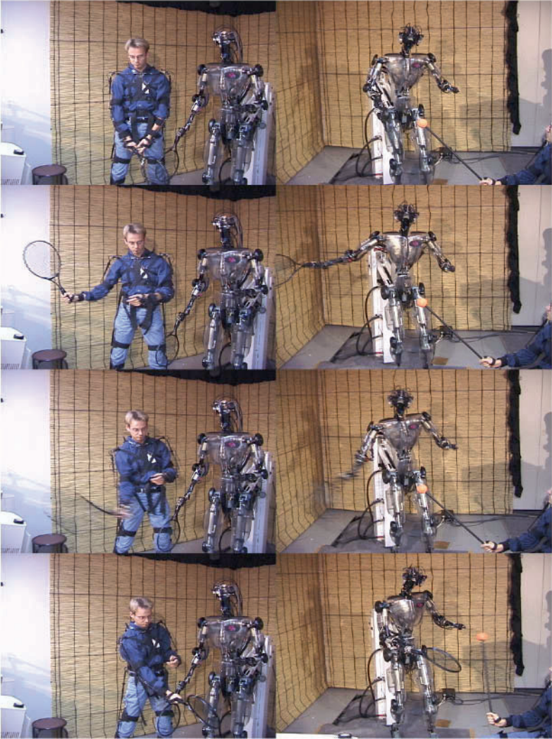
Fig. 3. Left Column: Teacher demonstration of a tennis swing, Right Column: Imitated movement by the humanoid robot.
