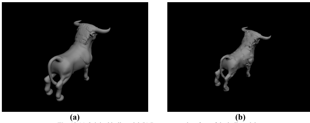
Fig. 13 (a) Original bull model (b) Reconstructed surface of the bull model.
