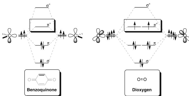
**Fig. 1** Qualitative molecular orbital diagrams for the alkene fragment of benzoquinone and dioxygen highlighting the key differences in their respective frontier orbitals
