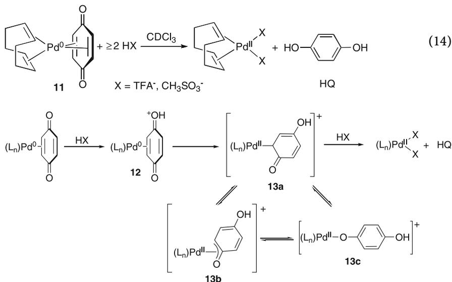
**Scheme 4** Mechanism of benzoquinone/acid-promoted oxidation of palladium(0)
