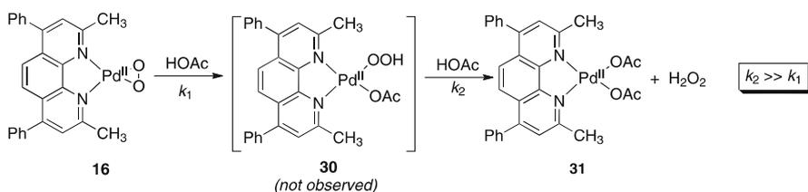
**Scheme 8** Protonolysis of (bc)Pd(O<sub>2</sub>), **16**, with acetic acid
