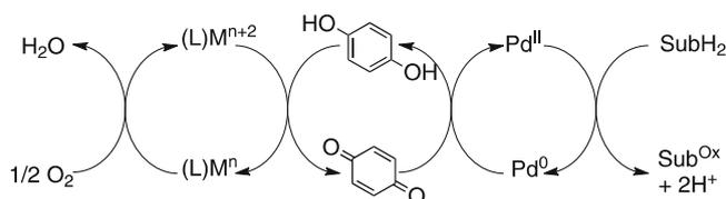
**Scheme 3** “Triple-catalysis” strategy for aerobic palladium-catalyzed oxidation reactions
