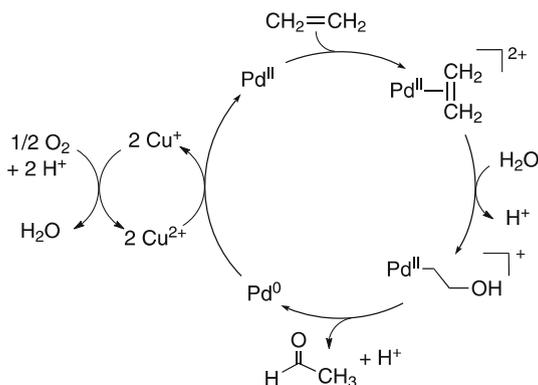
**Scheme 1** Catalytic mechanism for the Wacker process
