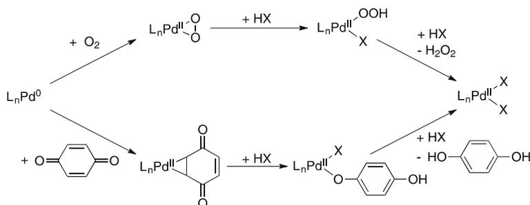
**Scheme 10** Mechanistic similarity between the oxidation of Pd<sup>0</sup> by dioxygen and benzoquinone
