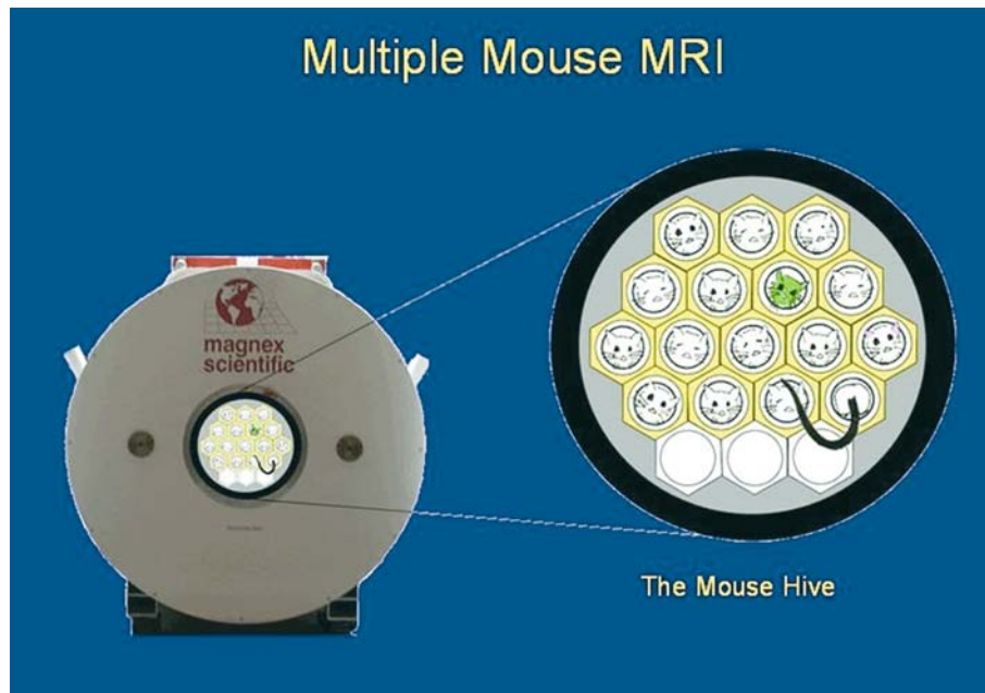
Figure 5. An MMMRI system for high-throughput mouse imaging. Nineteen independent transmit and receive coils share a common gradient and a 7 T magnetic field.
