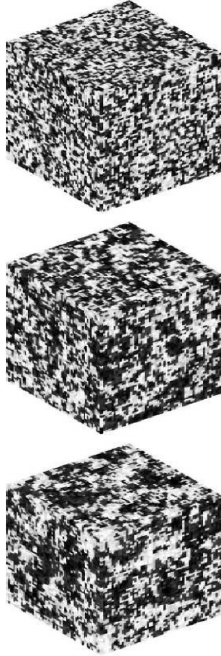
Fig. 2.24. From the numerical simulations in [15]: relative orientation \theta_i of the spins S_i in two copies ( a, b ) of a numerical Heisenberg spin-glass. The gray scale stands for \cos \theta_i(t_w) = S_i^a(t_w) \cdot S_i^b(t_w) . From top to bottom , three different waiting times t_w = 52, 27 , and 57\,797 s are represented, showing the slow growth of a local random ordering of the spins
