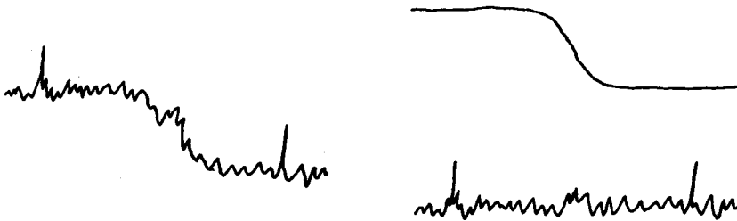
Fig. 1. A sequence of input property values (left) is modelled as a sequence of underlying values plus a pattern of fine variation (right).
