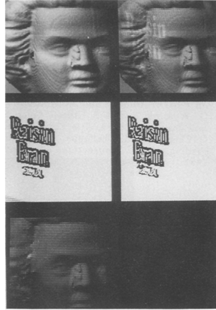
Figure 6. Mozart bust overlaid with color: (a) Intensity image. (b) Red chromaticity image. (c) Green chromaticity image. (d) (2nd row) Initial threshold. (e) Threshold after region-growing. (f) Output shading image. (g) (3rd row) Difference between (a) and (f).
