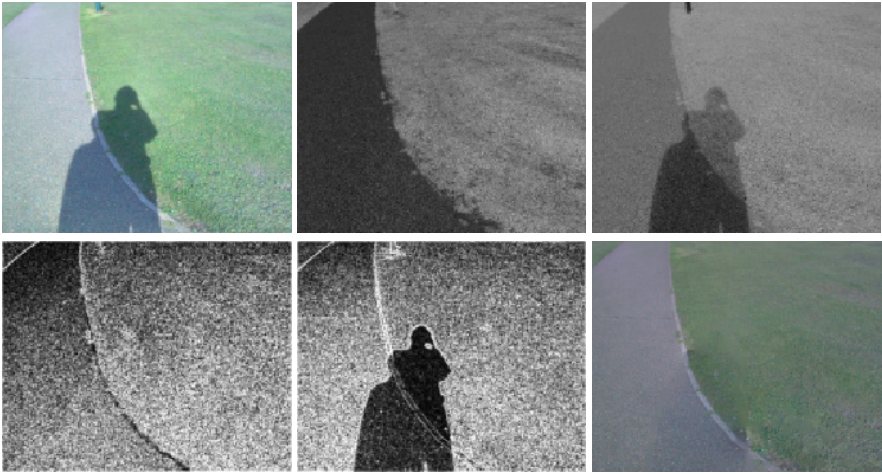
Fig. 1. (a): Original image. (b): Grey-scale illuminant-invariant image. (c): Grey-scale non illuminant-invariant image. (d): Edge map for invariant image. (e): Edge map for non-invariant image. (f): Recovered, shadow-free image.
