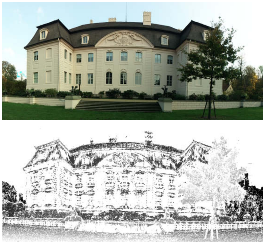
Fig. 5. Left image and disparity map of Branitz Castle. Disparity coding is the same as in Fig. 4. Matching window 7 \times 7 pixels, \alpha = 10 , \beta = 0.02 , disparity search range (0, 90), image size 2037 \times 4421 , 28% matched.
