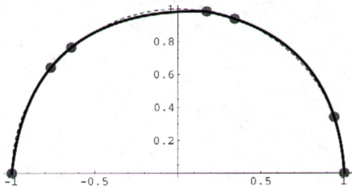
Fig. 2. Piecewise 4-point quadratic using 7 data points ( m = 6 ) from a semicircle (shown dashed). Length estimate: \pi - 0.00723637 .
