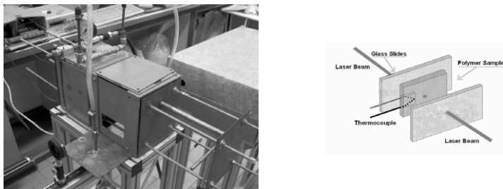
Fig. 16.2. Quenching device and sample assembly scheme
