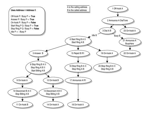
Fig. 2. CRESS Diagram for External View of SIP
