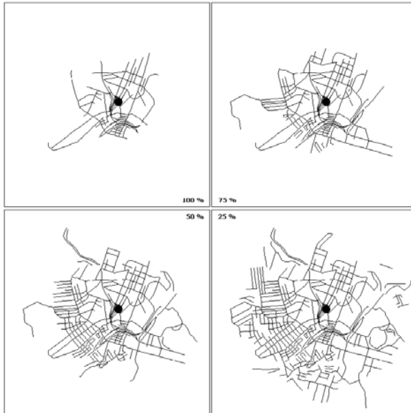
Fig. 7. Screenshot of the display threshold method used to visualize results of the query: “Find all Roads near a Specific Building (black circle)” for differing thresholds
