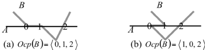
Fig. 8. Need for the order of characteristic points (where the orders of component types are same in (a) and (b), while the orders of their characteristic points are different)
