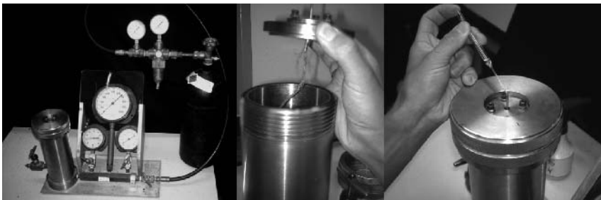
Fig. 17.1. Scholander pressure bomb. From left to right: Pressure bomb apparatus, inserting the root into the pressure cylinder, collection of plant sap from the root with a sterile Pasteur pipette
