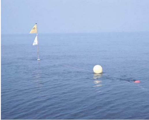
Figure 3. Surface markers of a T-POD mooring in the Baltic Sea
