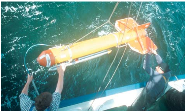
Figure 3. A sidescan sonar system was used (photo © Markus Diesing)
