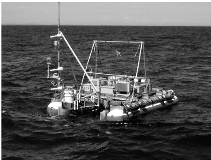
Fig. 1. Research catamaran during 1997 Coastal Ocean Processes experiment. The catamaran is shown here after deployment from R/V Oceanus in the North-western Atlantic Ocean. The platform is manoeuvred autonomously and is controlled remotely from the ship. During this experiment, the catamaran was equipped to measure long and short wave spectra, sub-surface turbulence, chemical enrichment, and various meteorological parameters. A system to measure vertical profiles of dimethylsulfide above the ocean surface was also incorporated into the catamaran measurement suite
